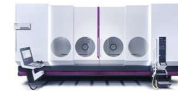
Y-Z travels Y 600 / 800 / 1000 mm - Z 1100 mm Tool holder (ZVH EXTREME) SK 50 • BT 50 • HSK 100
