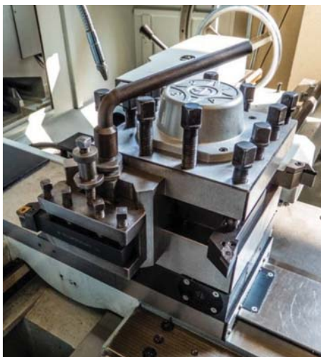
Optional adaptor to hold Q/C holders in position and manually change tools
