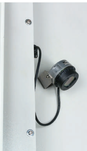
Heidenhain TT740+KHH100 (250) infrared probe for automatic kinematic measurement and calibration of 5 axis positioning
