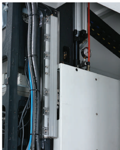
Optical Linear Scale X, Y, Z Heidenhain optical linear scales
