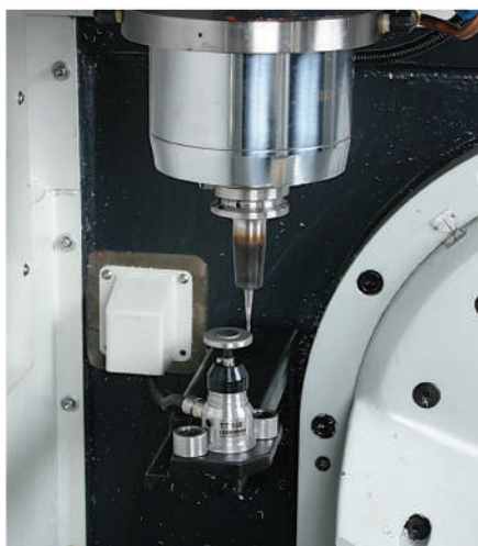
Heidenhain TT140 tool measuring system
