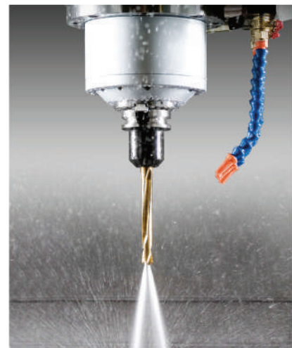
30 bar coolant through spindle system
