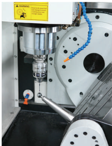
Heidenhain TT740+KHH100 (250) infrared probe for automatic kinematic measurement and calibration of 5 axis positioning
