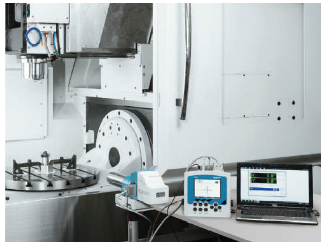
X, Y, Z, A, B axes are laser calibrated for linear positioning and angular accuracy
