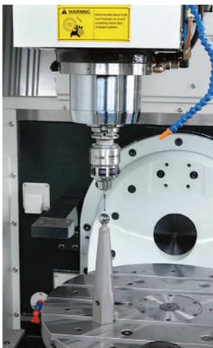
Heidenhain TT740+KHH100 (250) infrared probe for automatic kinematic measurement and calibration of 5 axis positioning
