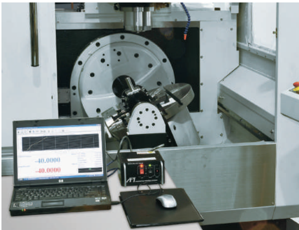
X, Y, Z, A, B axes are laser calibrated for linear positioning and angular accuracy
