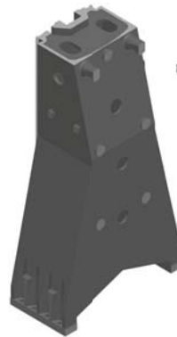
Inverted Y axis, one piece column structure
