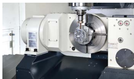
Positioning by worm and worm gear
