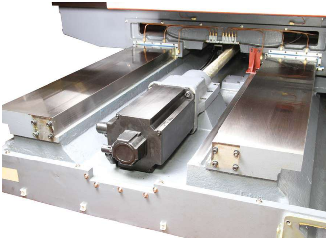
Heavy duty boxways available on Dugard HD Range
