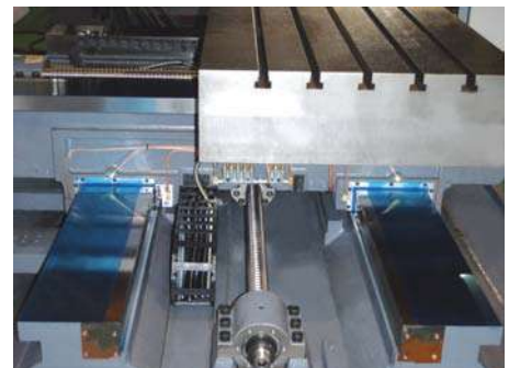
The sliding cover is wheel mounted so it will not damage the slideways
