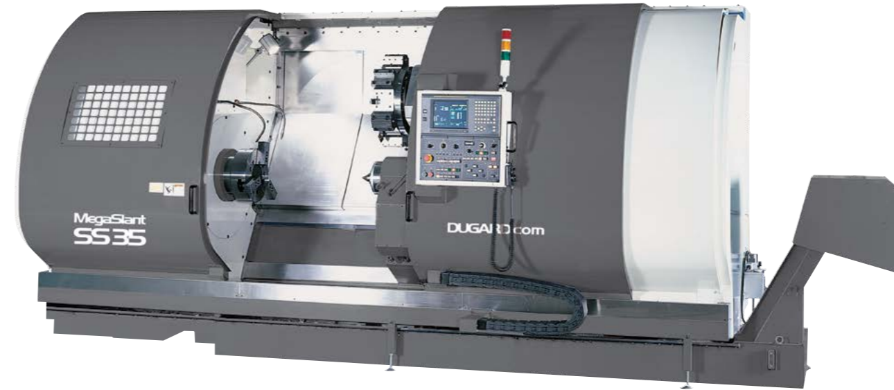
Bore 6" Centre distance 1,700mm
