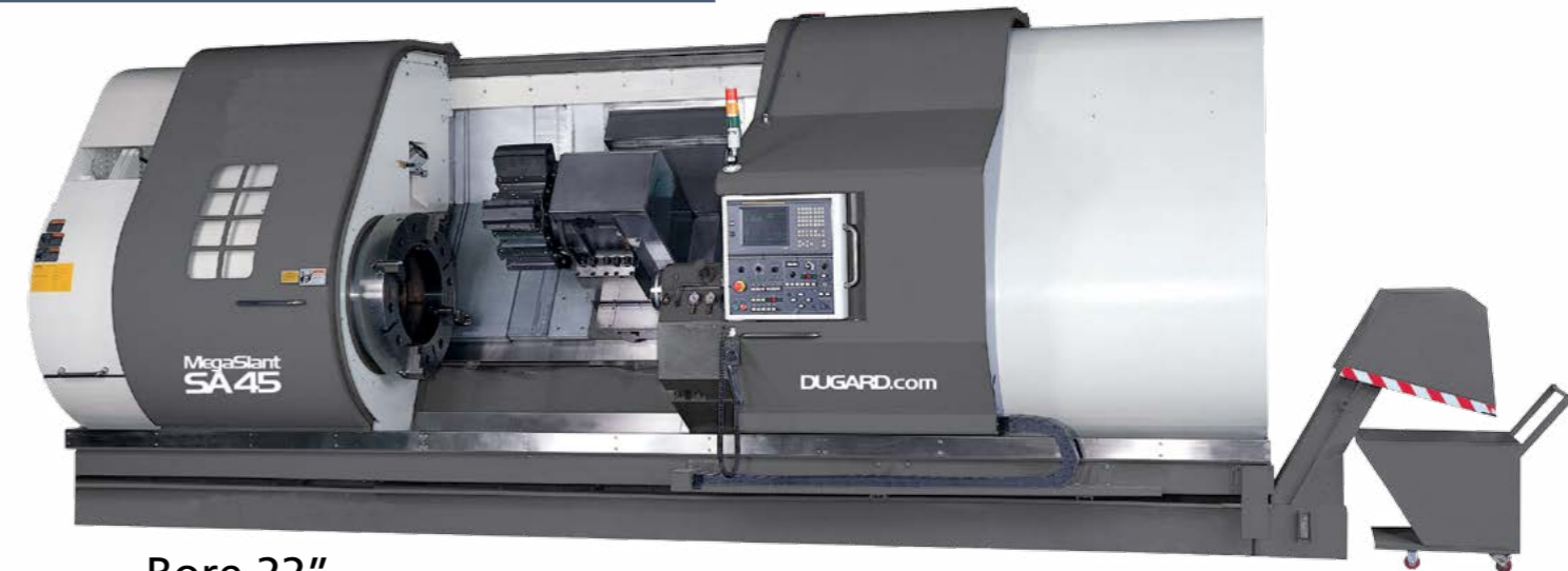
Bore 22" Centre distance 2,200mm Double Chuck
