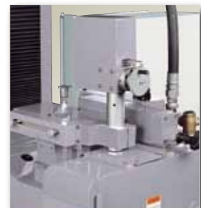
OVER-THE-WHEEL AUTO. STRAIGHT LINE DRESSING & COMPENSATION DEVICE B13-0406 (12 SERIES ) B13-0409 (16 SERIES )
