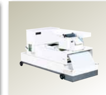
COOLANT SYSTEM WITH AUTO. PAPER FEEDING DEVICE & MAGNETIC SEPARATOR (WITH 1ROLL OF PAPER) B17-0302 Volume : 120L Paper feeding motor : 25W Pump : 1/8HP Coolant Capacity : 20L/min Space : 57"x24 3/8"(1450x620mm) Height : 30"(760mm)
