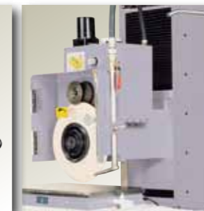
ROTARY DIAMOND DRESSER • B13-0306 (12 SERIES ) • B13-0307 (16 SERIES ) Rapid Elevating Power: 40W Dressing Power: 100W Auto Infeed: 0.00005" (0.001mm) Roller(optional): Ø4"x2"xØ1" (Ø100x50xØ25mm)
