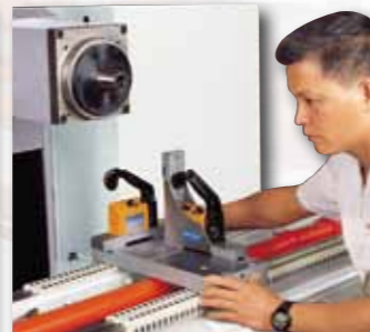
Driving force test on column
