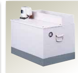
COOLANT SYSTEM WITH DOUBLE FILTER B17-0901 Volume : 95L Pump : 1/8HP Coolant Capacity : 20L/min Space : 26"x19"(660x480mm) Height : 24"(610mm)
