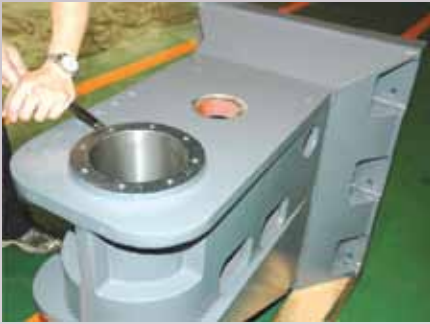
Precise head scrapping for spindle
