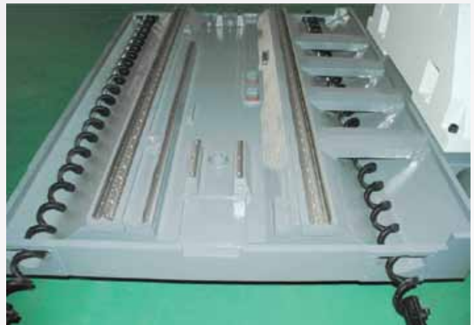
Broad base construction, dual type chip screw
