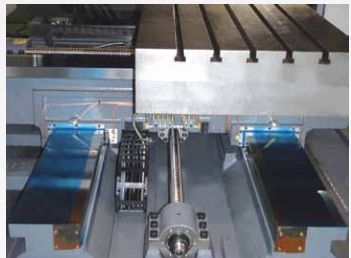
The rolling wheel of sliding cover does not damage the sliding trace
