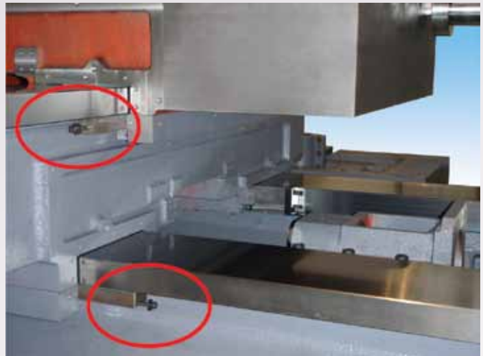
18 pieces of GIB on 3 axes avoid spindle head hanging down, saddle and work table swaying
