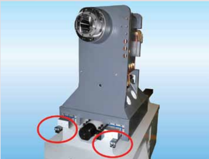
18 pieces of GIB on 3 axes avoid spindle head hanging down, saddle and work table swaying
